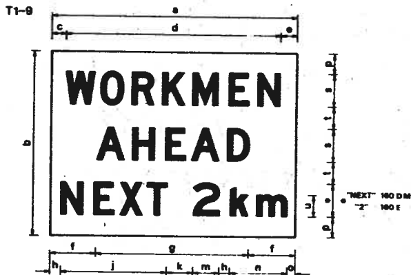
Black letters and numeral on fluorescent yellow-orange ground for day use Black letters and numeral on yellow reflectorised ground for night use
