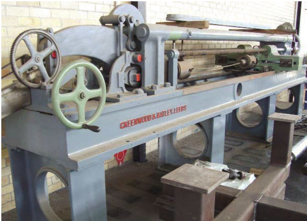
Figure 30: Greenwood and Batley Testing Machine at the University of Sydney
