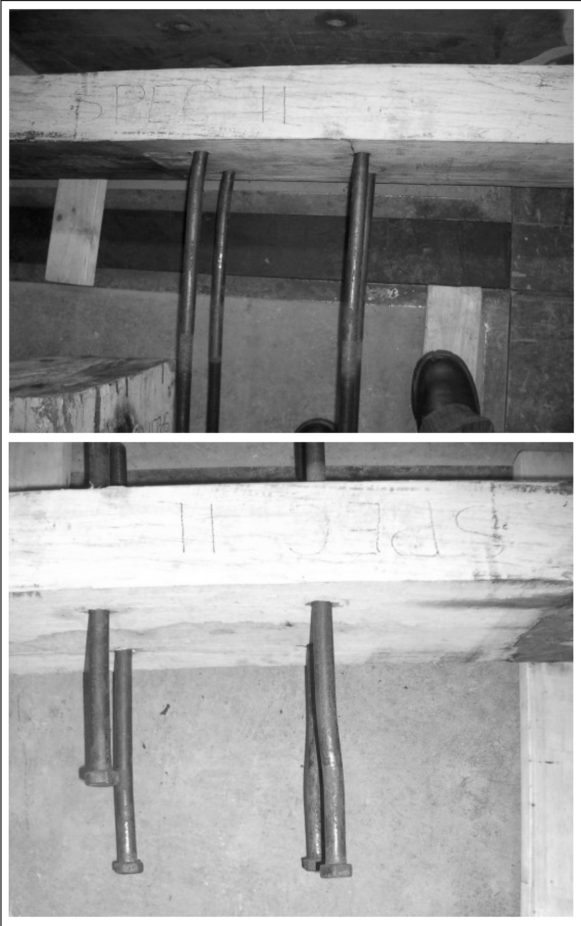
Figure 3.23: Photographs showing double curvature of one pair of bolts in Assembly 03-11
