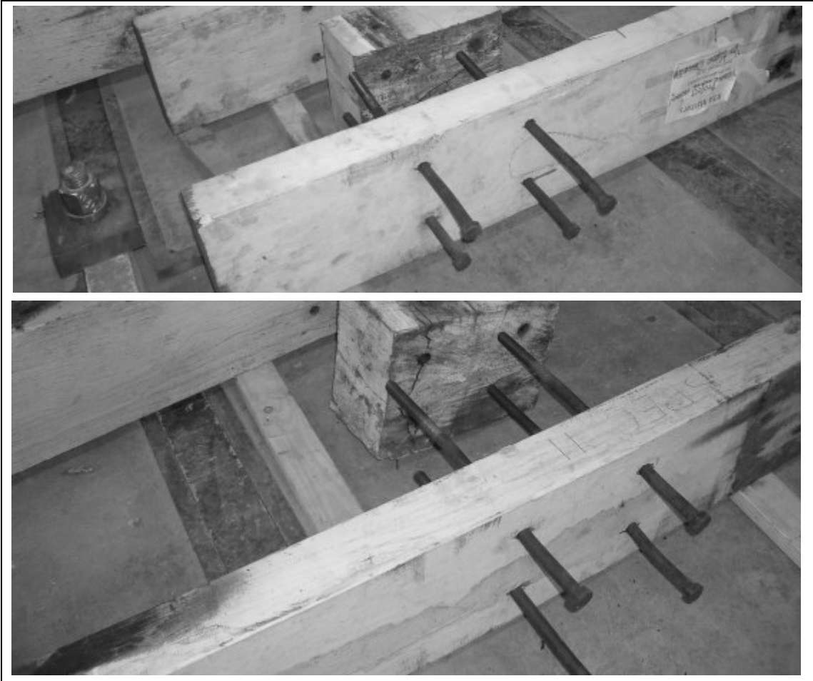
Figure 3.25: Photographs showing bolts after testing in Assembly 03-11
