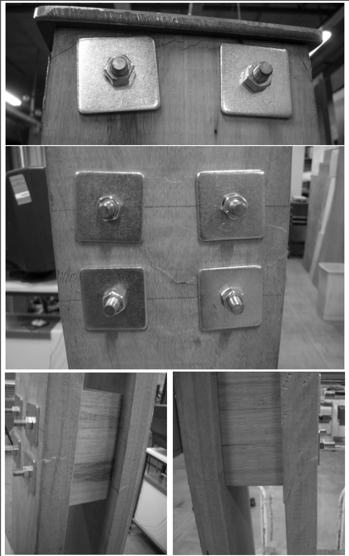
Figure A.5: Photographs of failure locations for Assembly 11B12A
