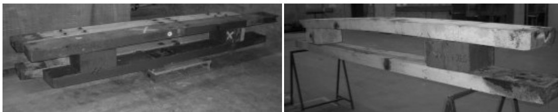
Figure 3.20: Photograph before bolting of assemblies 05-07 (left) and 02-09 (right)
