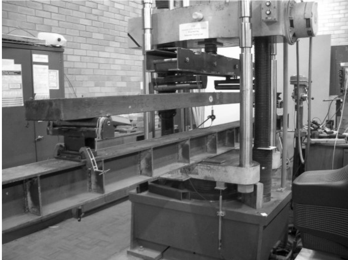
Figure 3.9: Photograph of Modulus of Elasticity testing for timber from Tabulam Bridge
