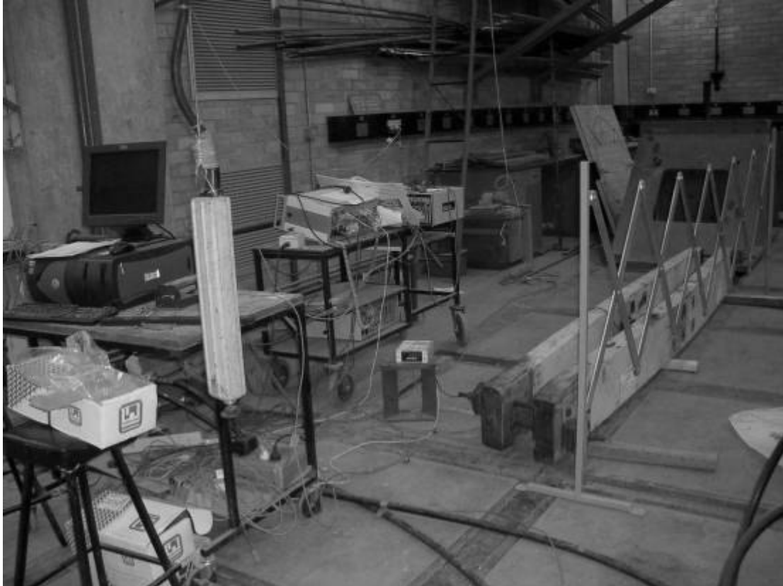
Figure 3.14: Photograph of 45 Day Constant Deflection Creep Test
