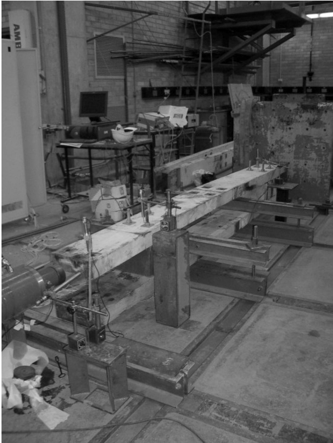
Figure 3.21: Photograph showing setup for shear test
