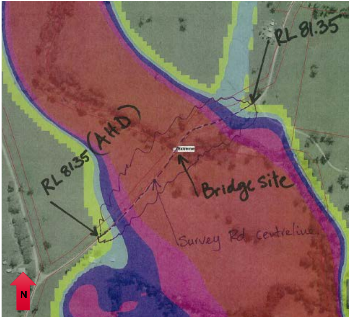
Figure 6-2: Flood study results for Monkerai Bridge.
