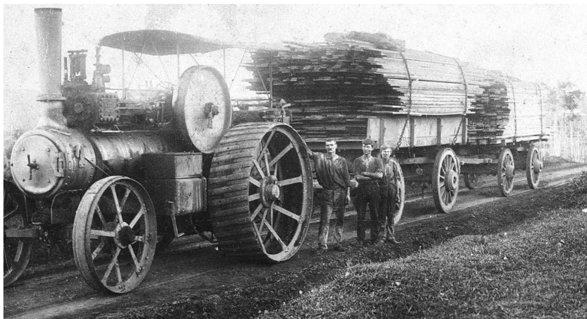
Figure 3.13 Steam Traction Engine hauling sawn pine from Dorrigo along the Bellingen Road (Source: Collections of the State Library of NSW, call number 'At Work and Play – 01688')
