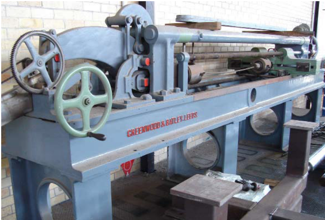
Figure 2-11: Greenwood and Batley Testing Machine at Sydney University.
